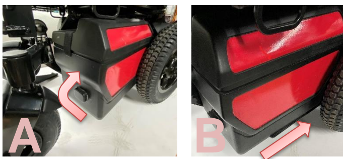
Figure 17: Replacing the boxes
