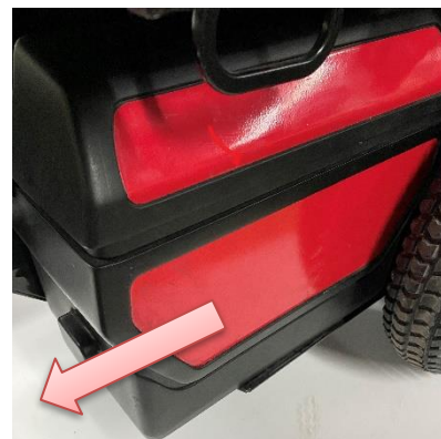
Figure 11: Remove battery boxes.
