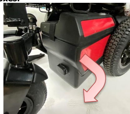
Figure 12: Remove battery box completely.
